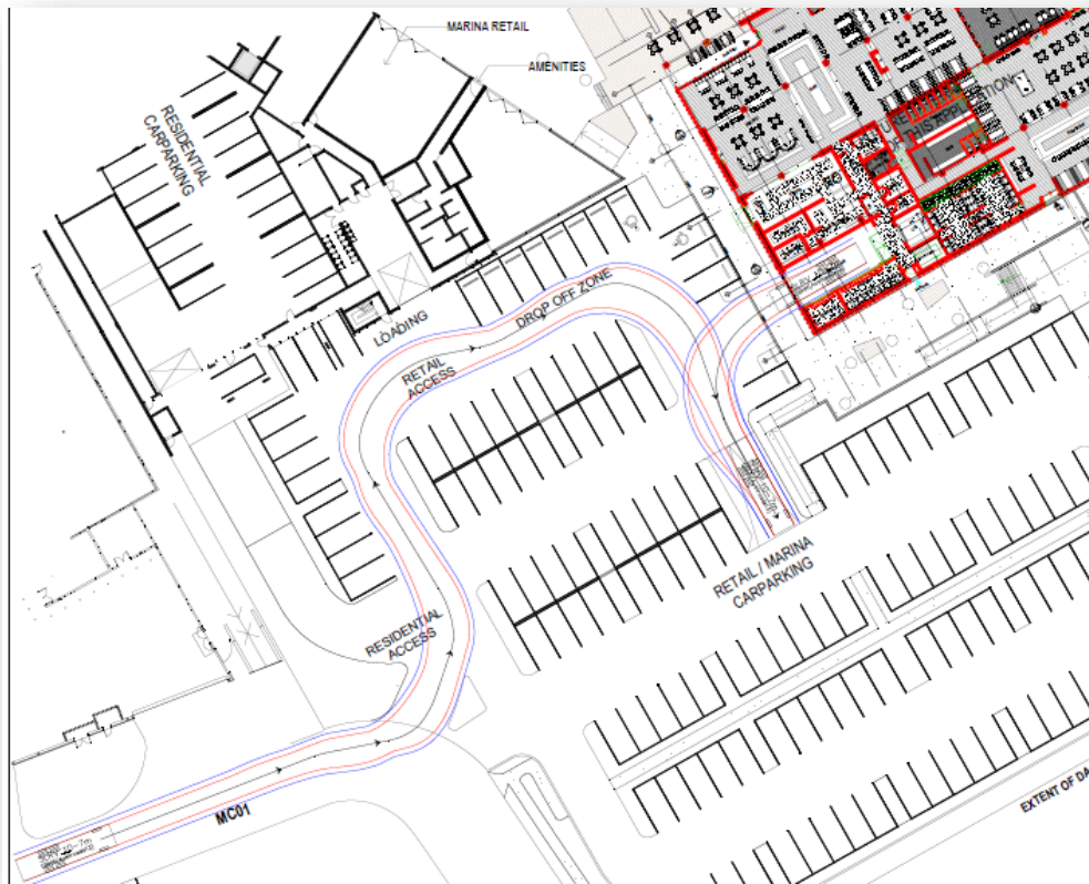
Figure 3 - swept path for 10.7 metre long rigid vehicle.
